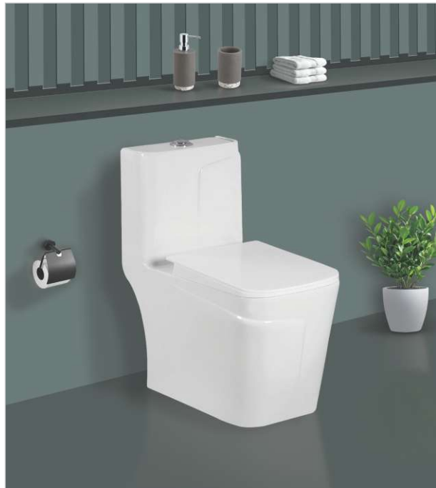
OP - 114 One Piece Closet 660 X 370 X 730mm Rimless, Washdown S-Trap : 225mm P-Trap : 180mm
