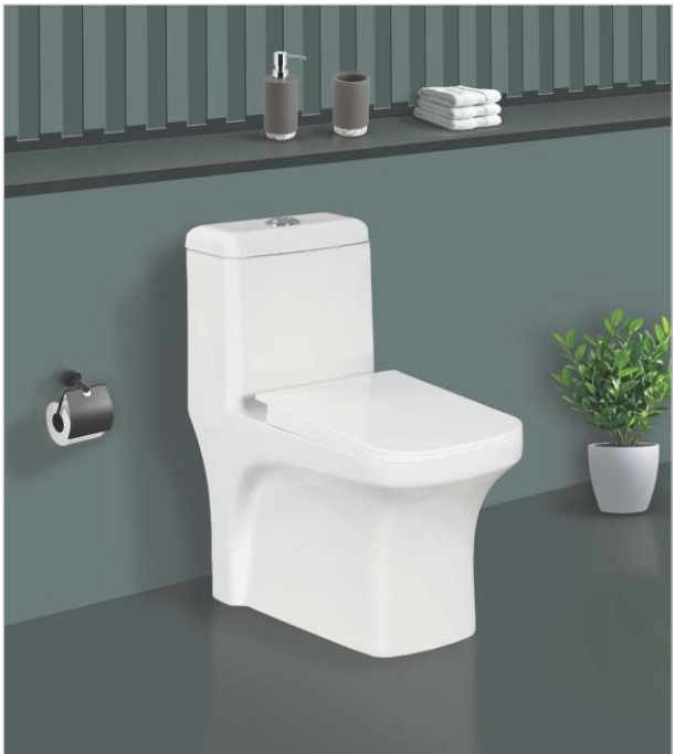
OP - 115 One Piece Closet 660 X 360 X 735mm Washdown S-Trap : 225mm P-Trap : 180mm
